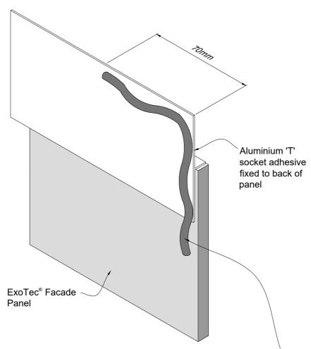
Apply 6mm diameter adhesive sealant bead to the back of the 'T' socket before fixing over ExoTec® main Top Hat section. Continue bead onto back of Panel. Install Panel before sealant cures to ensure bond.
